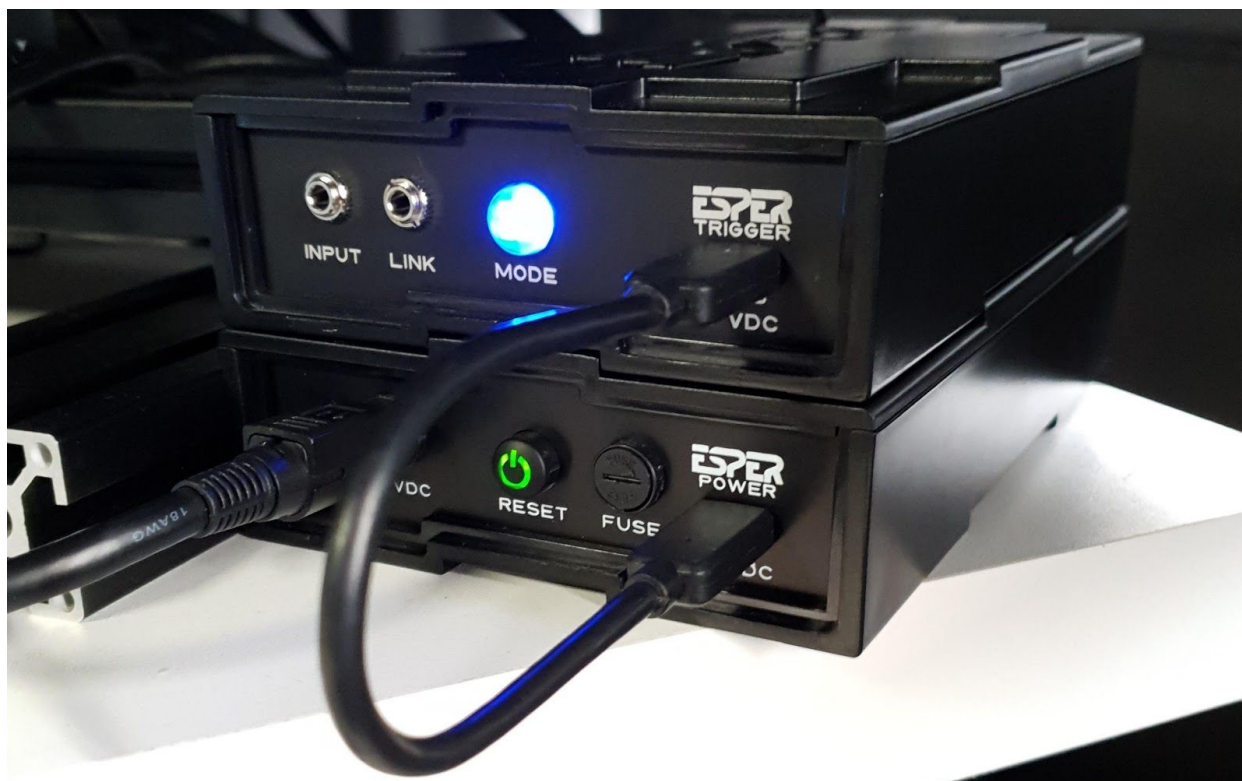
Figure 7. ESPER PowerBox powering the TriggerBox in 'Smart Trigger (Blue Mode)'
