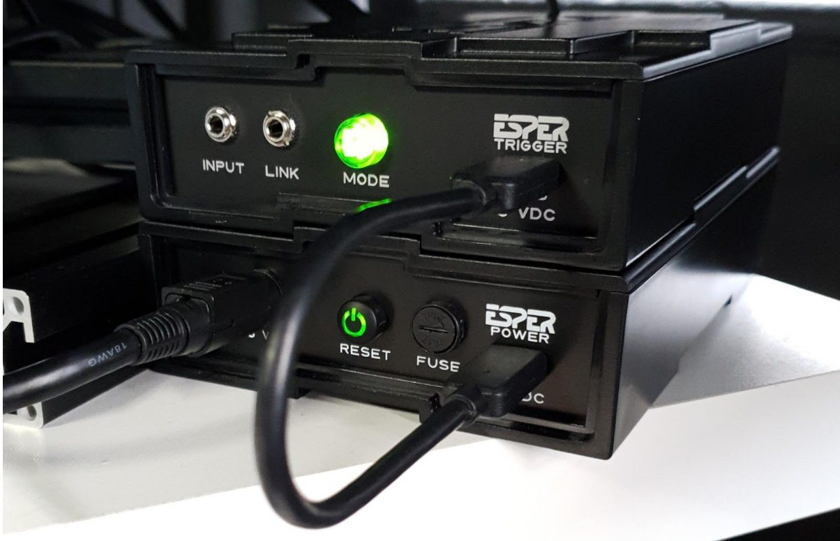
Figure 6. ESPER PowerBox powering the TriggerBox in 'All Trigger (Green Mode)'
